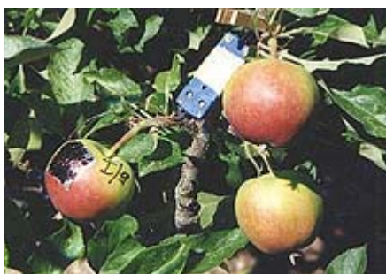
Fig. 2. Black patch method used to intercept solar irradiance and to heat peel of attached fruit in the field. A fine thermocouple attached to a psychrometric microvoltmeter was inserted under the black patch to measure peel temperature.
